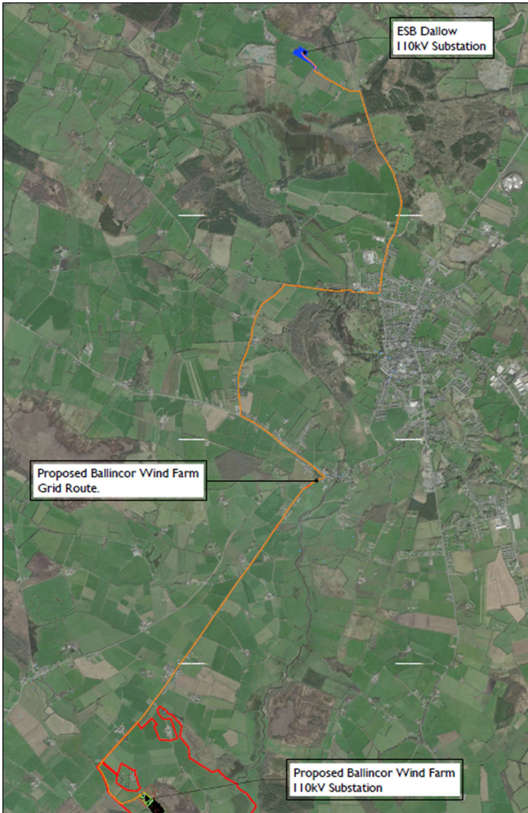
Figure 2.1: Map Indicating overall location of Ballincor Wind Farm and Grid Connection Route
